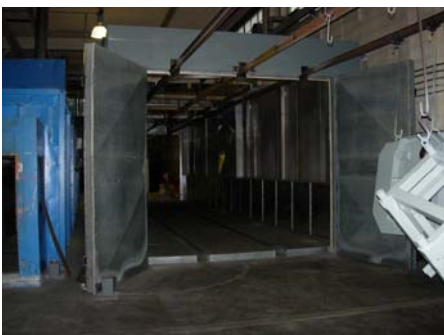
Pictured above is Northstar's 40 foot long oven which can hold a weight of 3 tons.
